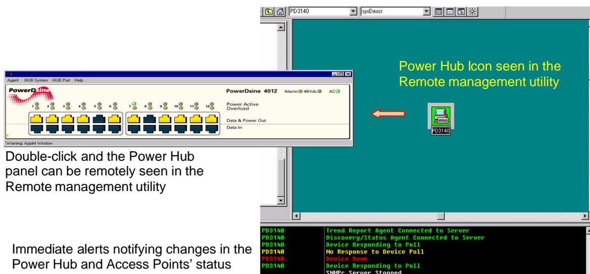
Double-click and the Power Hub panel can be remotely seen in the Remote management utility
